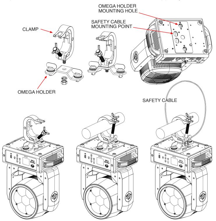
Screw one clamp via a M12 screw and nut into the Omega holder. Insert the quick-lock fasteners of the Omega holder into the respective holes of the adjustable mounting bracket. Tighten the quick-lock fasteners fully clockwise. Pull the safety-cable through the opening located on the bottom of the unit and over the trussing system or a safe fixation spot. Insert the end in the carabiner and tighten the safety screw.
