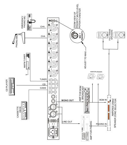
The above schematicillustrates a setup for a basic uninterrupted paging system.
