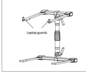
3. The stand can be set in Z position by adjusting the angle of the tray and legs, and turning the neck 180°.
