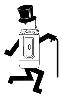
First up, placement. Don't extend past the operational range of 230 feet / 70 meters. By the same token, there should be a minimum of 10 feet / 3 meters between the transmitter and receiver. Additionally, allow as much line-of-sight as possible! Make sure there are minimal (or no) walls, heavy blankets, drapes or other barriers between the transmitter and receiver.
