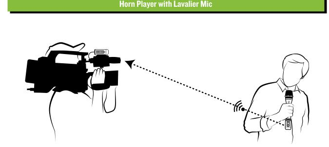
Here's another example that incorporates using a Mackie EM-89D mic that's connected to the EleMent Wave XLR transmitter. It is paired with its mate, the EleMent Wave receiver. As seen above, the belt clip of the receiver may be cold-shoe mounted to a video camera, camcorder or DSLR camera. Then an 1/8" cable is connected between the main output of the receiver and the input of the video camera. This is essentially the exact same type of setup that newscasters use.
