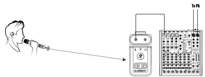
In this example, a Mackie EM-89D mic is connected to the EleMent Wave XLR transmitter. It is paired with its mate, the EleMent Wave receiver. An 1/8" cable is connected between the main output of the receiver and an open channel input of a mixer; a ProFX10v3 mixer, in this case. Then connect cables from the mixer's main outs to the PA system. It is the perfect setup for vocalists with great stage presence who like to roam the stage, presenters who don't want to be tethered by a cable and more!
