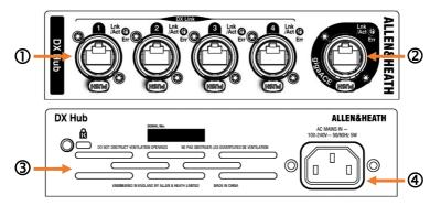
**D DX Link 1-4** Four DX Link sockets each capable of 32x32 channels of 96kHz audio. Each DX Link socket can be connected to 1 DX32 or up to 2 DX168/DX16-4W expanders. A status LED flashes yellow for Link activity and illuminates red to indicate a stream error.
