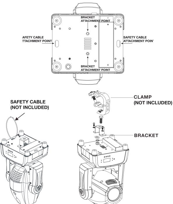
Screw one clamp via a M12 screw and nut into the bracket. Attach the bracket to the respective holes located on the bottom of the Focus Spot 2X. Tighten and secure the bracket screws. Pull the safety cable through the opening(s) located on the base plate and over the trussing system or a safe fixation spot. Insert the end in the carabine and tighten the safety screw.
