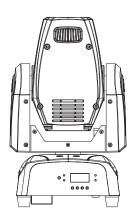
The Focus Spot 2X is fully operational in three different mounting positions, hanging upside-down from a ceiling or trussing, sideways on trussing, or set on a flat level surface. Be sure this fixture is kept at least 12m (40ft) away from any flammable materials (decoration etc.). Always use and install the supplied safety cable as a safety measure to prevent accidental damage and/or injury in the event the clamp fails (see next page). Never use the carrying handles for secondary attachment.
