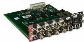
? ?????? Allen & Heath SuperMADI (M-DL-SMADI-A) ??????? 128 ???????? / ??????? ??? 96kHz ? 48kHz ?? BNC connectors ? optical (SFP ??????). ????? ??????? ?? ?? ????? dLive.
